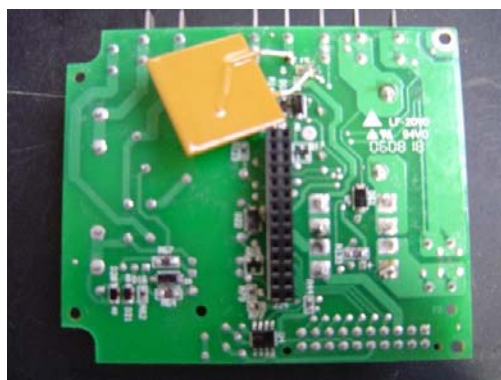
Modified power board with re-settable fuse shown in position
