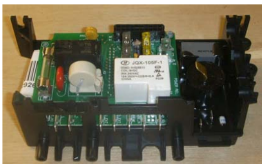
Power board old version Underside of Top Half F5 fuse is at top centre
