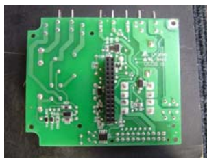
Power board old version Underside of Top Half F5 fuse is at top centre
