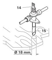
Install the safety/drain valve (14) at a place which is easily accessible, near the water heater. Drill hole with 18 mm diameter and pass through discharge socket with hose (15). Fasten safety/drain valve with 2 screws. The draining is to be directly to the outside at a position protected against splash water (apply splash guard, if necessary).
