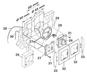
If it is not possible to install the control panels flush with the surface, Truma can provide a surface-mounting frame (25) on request, as a special accessory (part no. 40000-52600).
