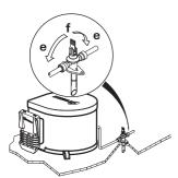
e = Lever position "Closed" f = Lever position "Drain"
