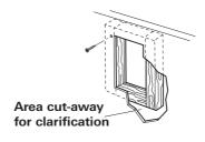
If there are any cavities in the area of the cowl, pack these with pieces of wood so as to be able to tighten the screws. The finished hole should be 168 mm high and 92 mm wide.
