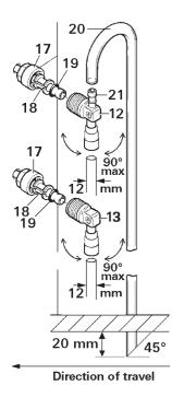
2. Screw elbow with integrated breather valve (12) to hot water connection pipe (upper pipe) and elbow without breather valve (13) to cold water connecting pipe (lower pipe).
