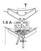
Only replace the miniature Fuse on the p.c.b. with a fuse of the same type: 1.6 A, EN 60127-2-3 (slow action).
