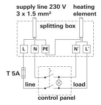
Cables must be in accordance with the technical rules and regulations of the country in which the vehicle is to be registered, for the first time.
