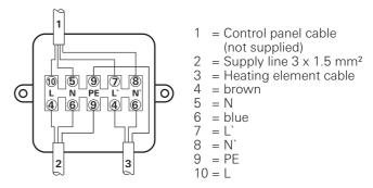
2. Assemble the splitting box on the vehicle floor or on the wall, in the vicinity of the appliance (observe heating element cable length 110 cm!).
