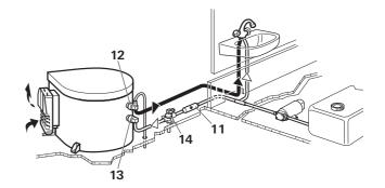
When using the Truma Ultrastore together witch the Truma Ultraflow pressure switch, the use of a non-returnvalve is essential (please refer to the pressure switch instruction).
