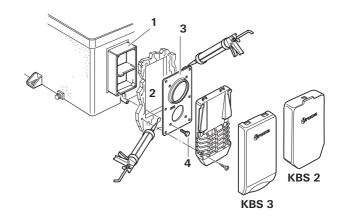
4. Remove sealing frame (3) and coat with non hardening mastic on the side facing the vehicle – do not use silicone!
