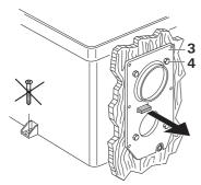
Screw the sealing frame (3) in contact together with the cowl body (1) so the anti-twist device projects out!
