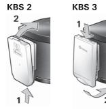
Before setting off on any journey, fit cowl cap KBS 2 or KBS 3 with the boiler switched off. Please ensure that it is secure and has locked into place (risk of accident). Defective cowl caps must not be used.
