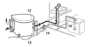
When using pressure pumps with high switching hysteresis, hot water may flow back through the cold water tap. To prevent the backflow, we recommend that a non-return valve (11 – not included in the scope of supply) be fitted between the outlet to the cold water tap and the drain valve.
