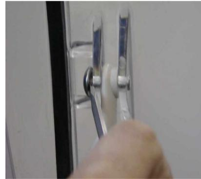
2.) Remove the cap by using a screwdriver.
