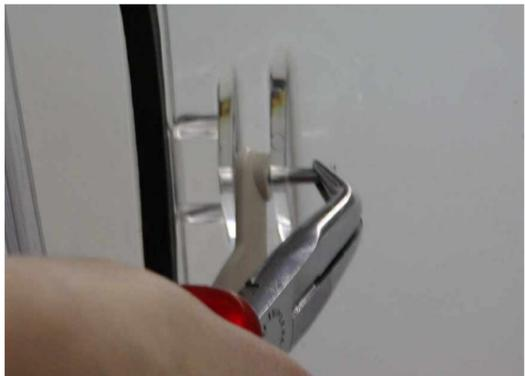
3.) Remove the bolt with a pointed plier.
