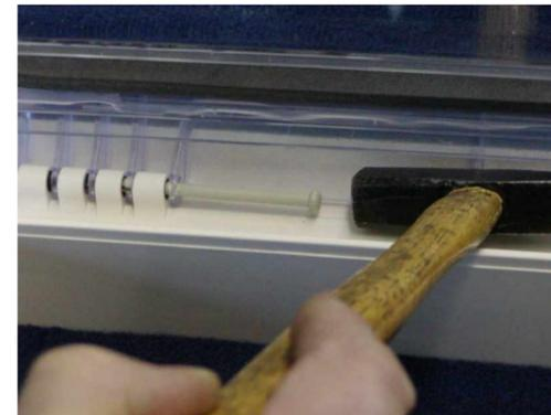
9.) Beat the hinge-pin into with a hammer.
