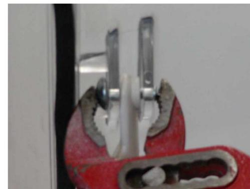
11.) Press the cap with a tong to the bolt.
