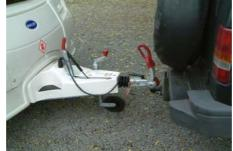
Lower the jockey wheel to the ground and clamp in position. This is to assist with weight distribution when the wheel is lifted.
