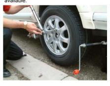
Locate the replacement wheel onto the brake drum and fasten wheel bolts finger tight. Using a torque wrench, torque up the wheel bolts to the manufacturer's recommended setting in the correct sequence i.e. North, South, East and West. Remove the axles stand (if used), raise the corner steadies, raise jockey wheel and release the handbrake.
