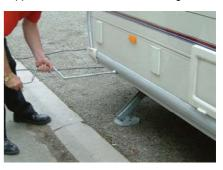
Use the AL-KO corner steady brace to lower the corner steadies on the same side as the wheel to be changed. This is to assist stability of the raised caravan. DO NOT use the corner steadies to jack up the caravan. For additional safety we recommend the use of an axle stand, if available.
