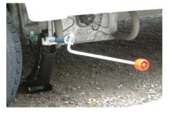
Position the AL-KO side-lift jack into the jack brackets. Raise AL-KO side-lift jack sufficiently to allow the wheel to be removed, and the replacement wheel to be fitted.
