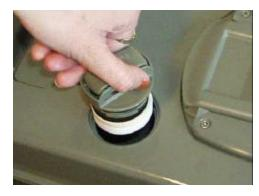
2. Split the automatic vent in the two main parts: the green/grey button and the white foam part. To do this, you'll have to push in the green button and at the same time push with your other hand against the white foam (A). Carefully move the parts until you feel the thin pin, which connects the two main parts, coming out of its setting. Now you can carefully pull the pin from the green/grey part (B).
