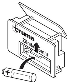
Only use temperature resistant (+70° C), leakproof Mignon batteries (LR 6, AA, AM 3, part no. 30030-99200), other batteries could cause operational faults!
