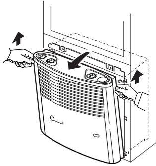
Then move the front case aside so that any connecting cables (e.g. for the Piezo-igniter, the warm air fan and the ignition indicator lamp or the open fire) do not have to be disconnected.
