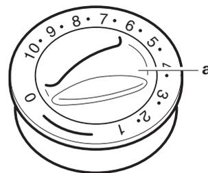
3. Keep the control knob pressed down for a further 10 seconds to allow the safety pilot to operate.
