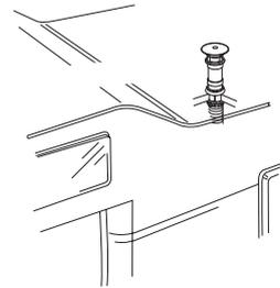
The camper manufacturer or heater installer must perform test drives to determine the combination of cowl top and extensions (if required) for the individual as delivered vehicle configurations and consult Truma if necessary. Depending on the vehicle model and the equipment installed on the roof, cowl top T1 (part no. 30700-01) or T2 (part no. 30700-02) may be required.
