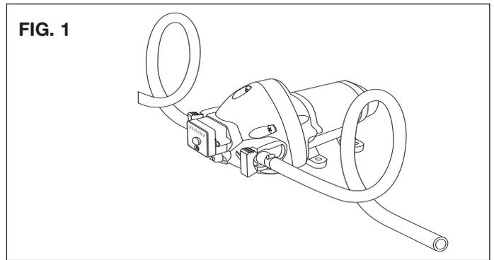
**Note:** To help reduce noise and vibration of the pump through the system use flexible lines on the inlet and outlet of the pump as shown above. Be sure to use lines rated to not collapse under pump vacuum.
