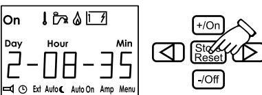
If the power to the panel is broken and the battery backup is not connected, the clock must be set again.
