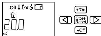
The pump is in automatic position. The lower menu row is not lit up.
