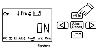
When you get to the vehicle and AutoOn is activated, de-activate AutoOn so that the heater does not stop after 24 hours (the boiler cannot be switched off when AutoOn is activated).
