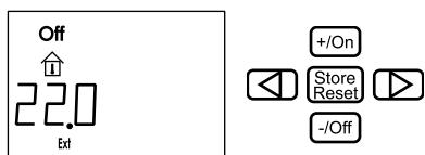
When external start is activated the heater will start with the latest settings and "ON" (main breaker) comes on. If 12V is not connected to the heater, the display will not light up until 12V is connected. The external start function is still activated.
